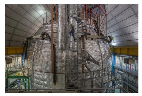
Figure 4.12: The figure shows the detector after thermal insulation<sup>1</sup>.
