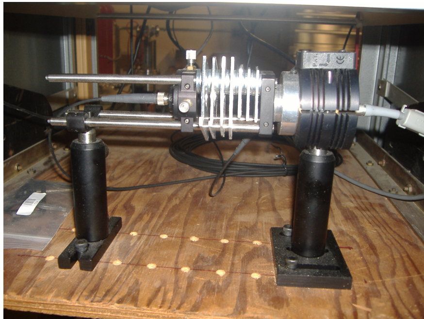
Figure 4.6: Photograph of the diode laser, filters, and optical fiber used to calibrate the PMT response.
