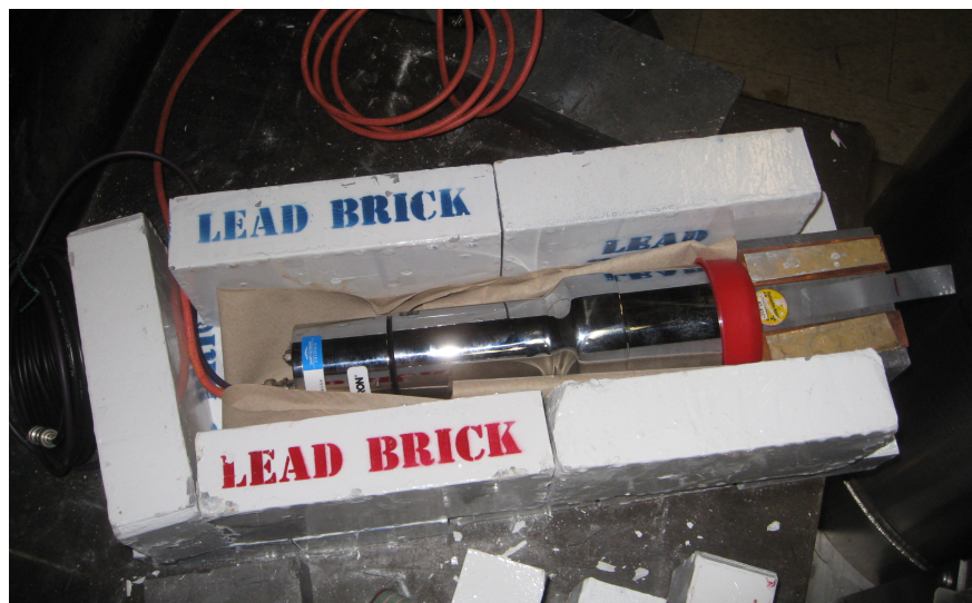
Figure 4.51: Photograph of the external NaI detector and shielding, set up for a collimated ^{22}\text{Na} coincidence measurement, with the top layer of shielding removed.
