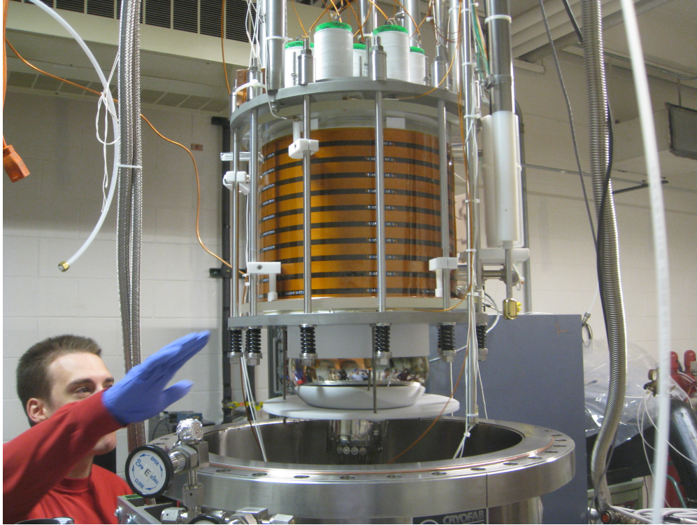
Figure 4.2: Photograph of the 10kg prototype inner detector during assembly.
