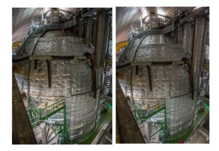
Figure 17: Pictures of the Borexino detector water tank covered with the insulation layer, in the left picture it is covered partially, and in the right one totally covered.
