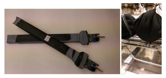
Fig. 3.3: The external muon tagging system through plastic scintillators coupled with SiPMs.
