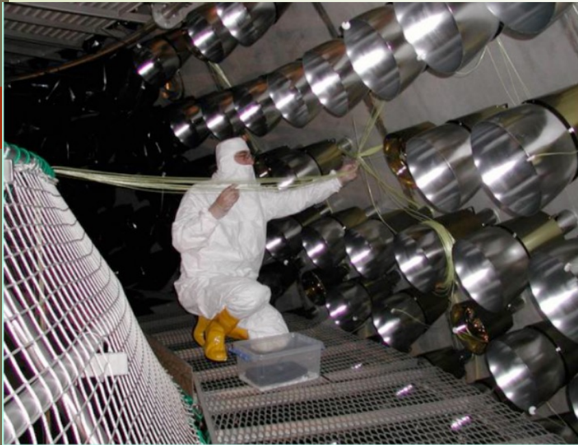
Installation of the optical fibers- Lino (Barbara)
